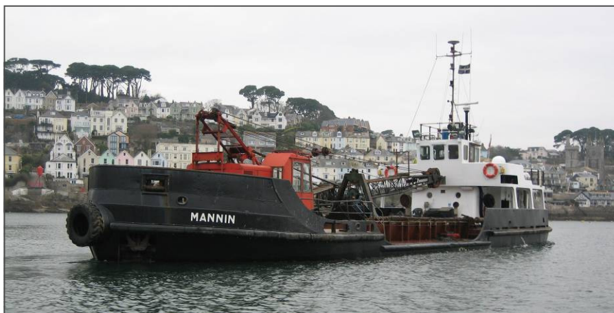
Grab Dredger 'Mannin' in Fowey
